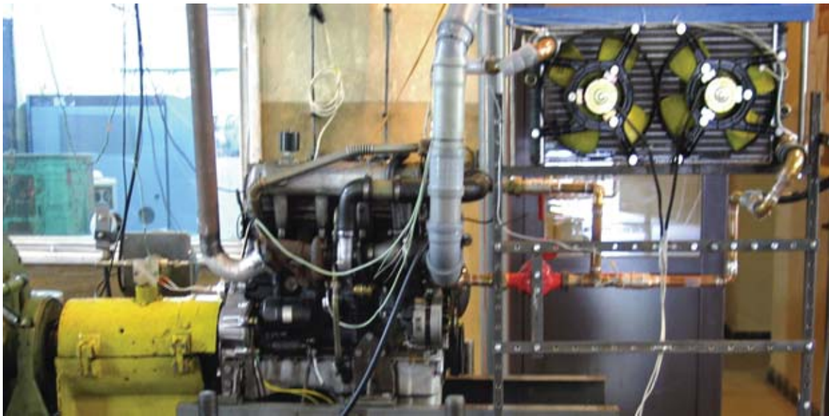
Fig. 3. Schema of the cooling system (a) and view of the engine with this system (b): 1 – fan controller, 2 – trim tank, 3 – radiator, 4, 5, 6 – valves, 7 – manometer, 8 – engine, 9 – water pump, 10 – water flow meter
